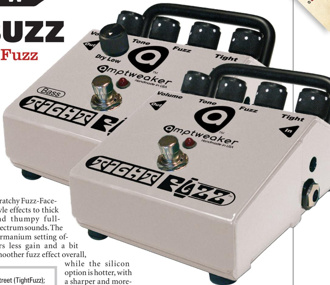
Adding to the versatility of both pedals are built-in effects loops with pre/post (fuzz) switches. We tried a number of effects into each, including an overdrive (which really ramped up the fuzz and sustain), and an envelope filter that produced fuzz reminiscent of an E-H Bassballs box. The loop is engaged only when the fuzz effect is, so both can be turned on with one stomp.
